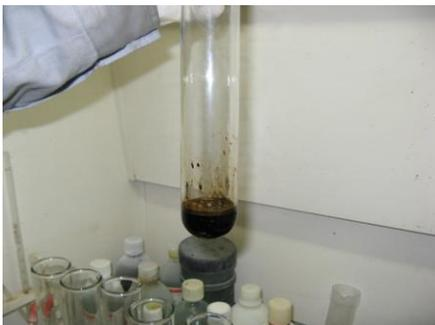
12. Cool and dilute to 50 ml with reagent water. The sample is now ready for analysis for TKN and TP.
