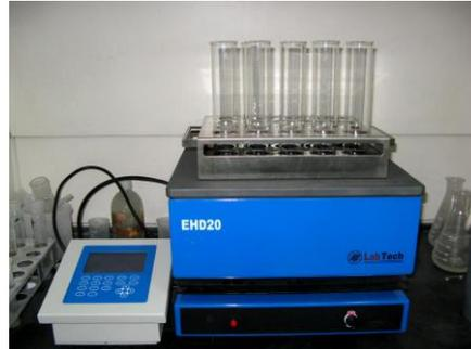
8. Set the digestion temperature on 160 °C.
