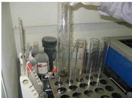
3. Add 0.2g  $\text{CuSO}_4$  and 3g  $\text{K}_2\text{SO}_4$  to the sample tube.
