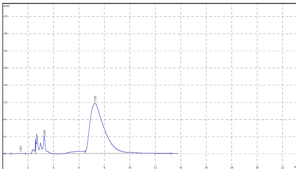
Figure 2 Chromatogram of standard clenbuterol (1.0 $\mu$ g/mL)
