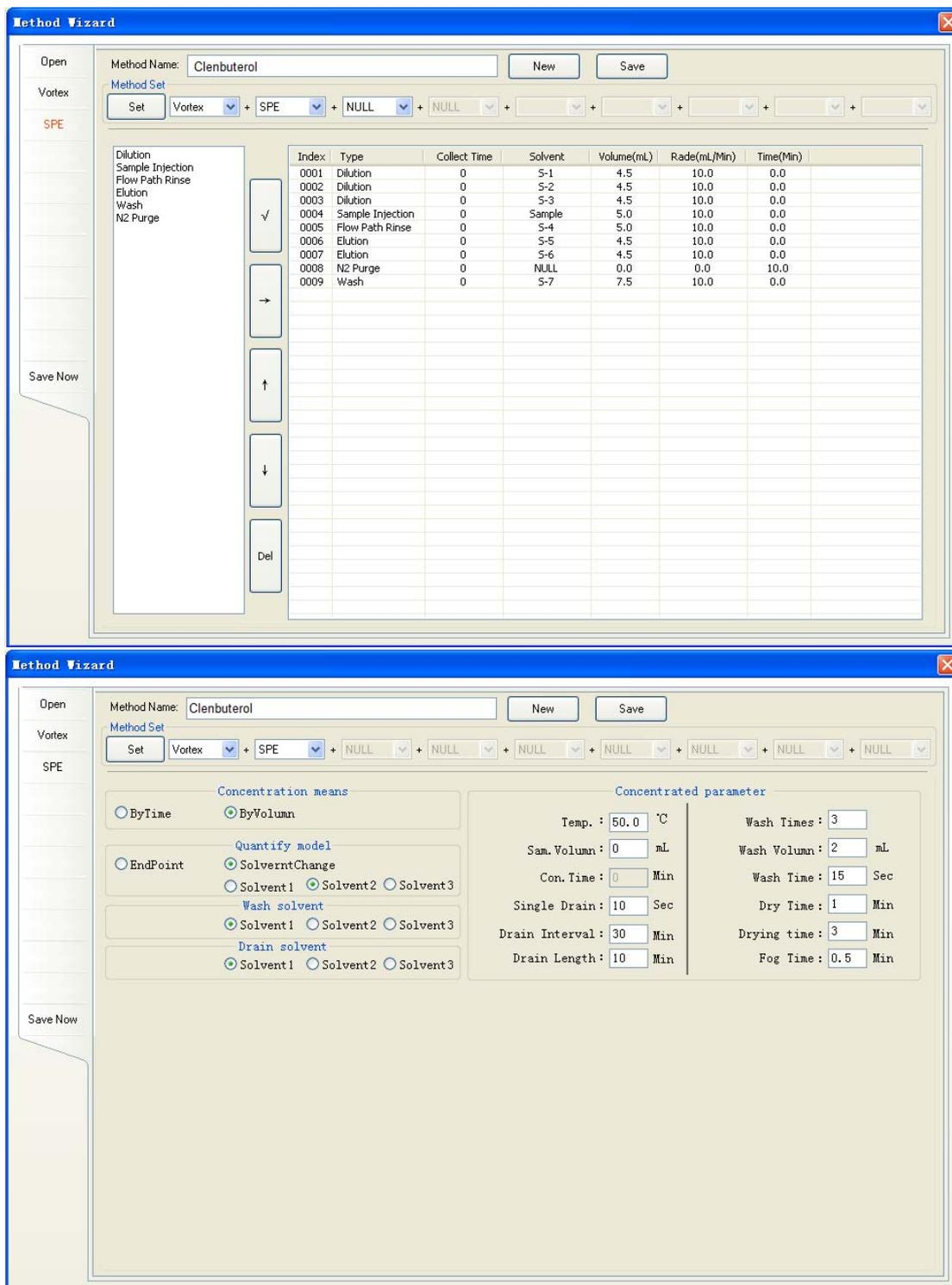
Figure 1 Method setting interface for PrepElite-VS
